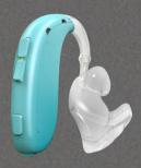
Oticon Xceed Play BTE UP is a ultra power hearing aid with a 675 battery. The style has separate push buttons for programs and volume for easy usage and control. It features T-coil, optional LED indications and support for class room systems.
